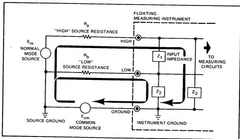
FIGURE 4. Inside an Ideal Floating Voltmeter
