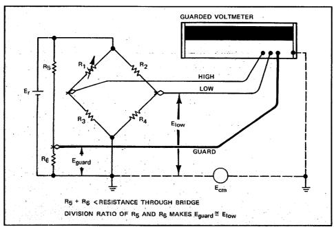
FIGURE 10. Driving the Guard in a Bridge Measurement
