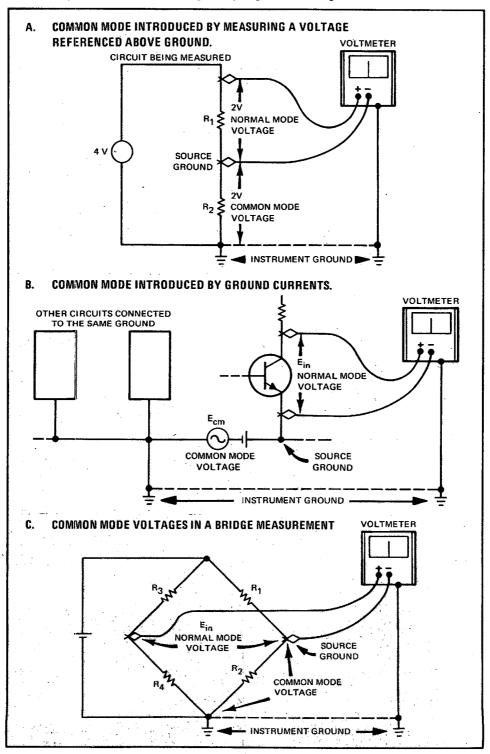
FIGURE 3. Some Examples of Floating Measurements
