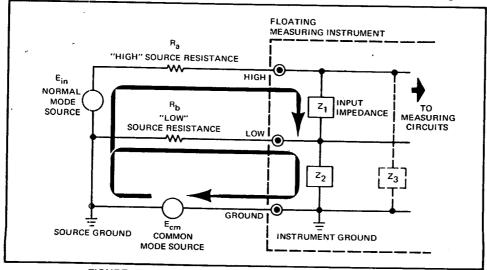
FIGURE 5. A More Realistive View of a Floating Voltmeter
