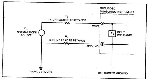
FIGURE 1. Simple Grounded Measurement
