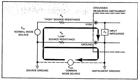
FIGURE 2. Grounded Measurement with a Common Mode Voltage
