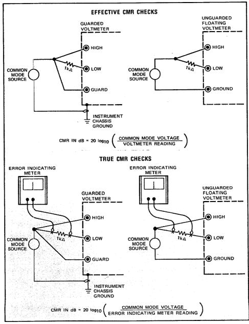
FIGURE 13. Common Mode Rejection Checks
